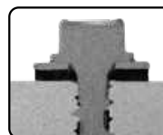
KS V-Neck Anatomy of the KS V-neck weather tight system
