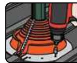
5. Fasten Retrofit to roof
